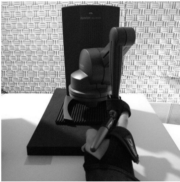
Fig. 2. Illustration of the haptic device. The participant's right index finger was strapped into the haptic device.
