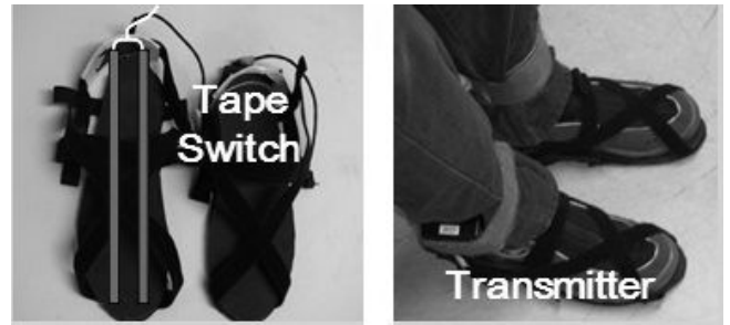
Fig. 2. Devices of experiment. Foot switches were in these devices, and all participants wore these devices while gait measurement.
