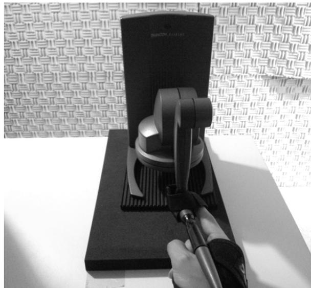
Fig. 2. Illustration of the haptic device. The participant’s right index finger was strapped into the haptic device.
