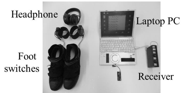
Fig. 1. Device for gait training using rhythmic auditory cue.
