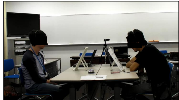
Fig. 2. Snapshot of experiment environment. Two digital video cameras capture the participants, two laptop with headsets record real-time vocal data, and accelerometers attached to forehead and body of participant record real-time head and body motion data.
