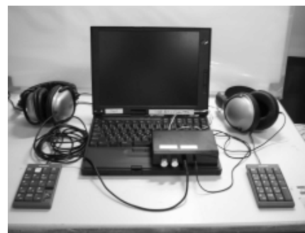
図3 協調タッピング装置 Fig. 3 Equipment of cooperative tapping system
