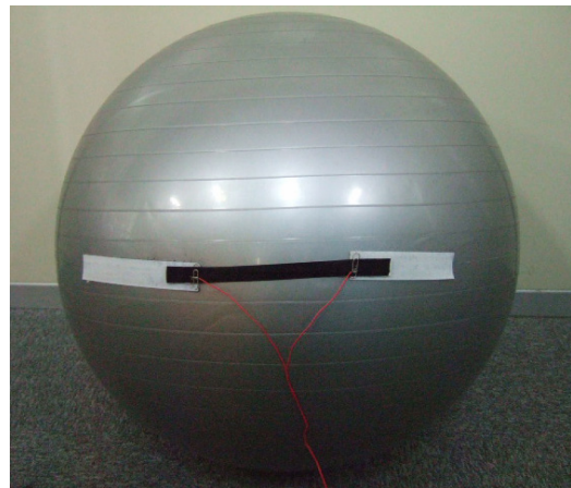
Fig.3 導電性ゴムの取り付け Fig.3 Installation of electroconductive rubber to exercise ball
