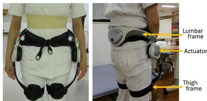
Fig.1 Walking assist device
