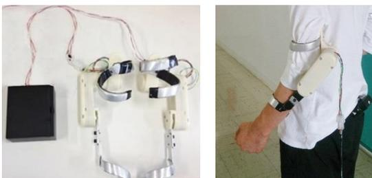
Fig.1 Elbow driving device
