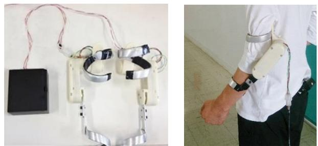
Fig.1 Elbow driving device
