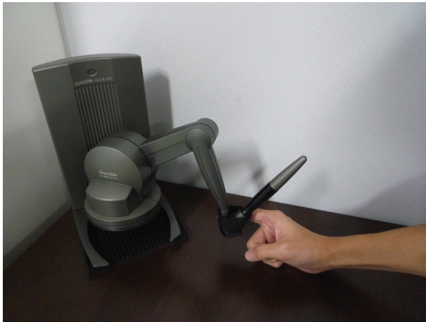
Fig.1 Haptic stimulus (3[N], 15[ms]) was presented to participant's right hand by Haptic Device.
