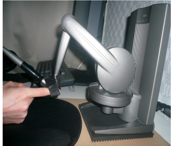
Fig.2 The device to present tactile stimuli and to move participants' arms.
