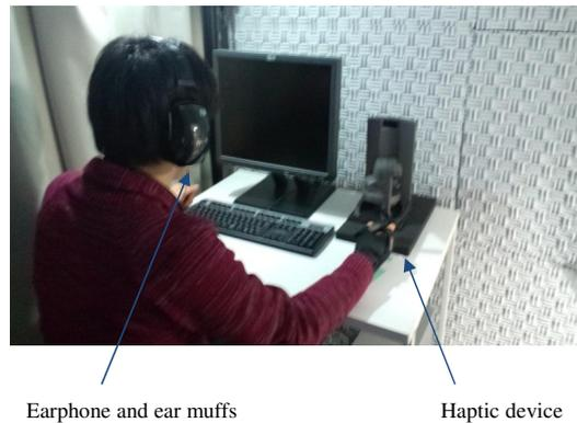
Fig.1 The experimentation environment. Sinusoidal wave sound was presented through earphone. Haptic device was attached with participant's right index finger. Under the Involuntary condition, the haptic device moved participant's finger.
