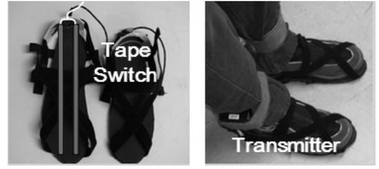
Fig.2 Device of experiment. Foot sensors were in these devices, and all participants wore this device while walking measurement.
